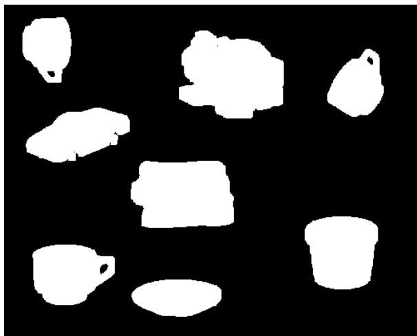
(c) After opening by a 5x5 square, there is no more noise and object's contour are a little bit better
